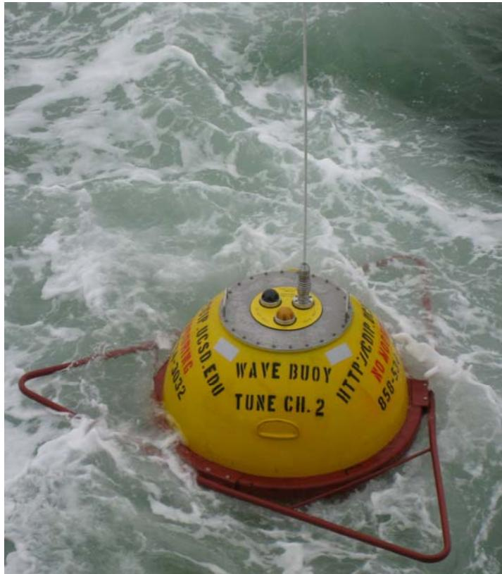
Buoy measures wave height, wave direction, wave period and sea surface temperature.
